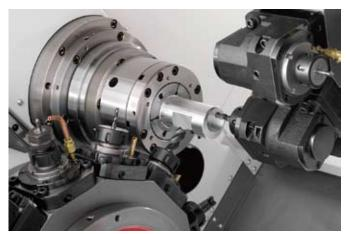
Simultaneous complex machining with two turrets
