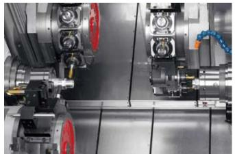
Simultaneous complex machining with three turrets
