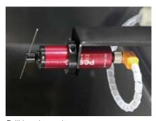
Drill breakage detector
